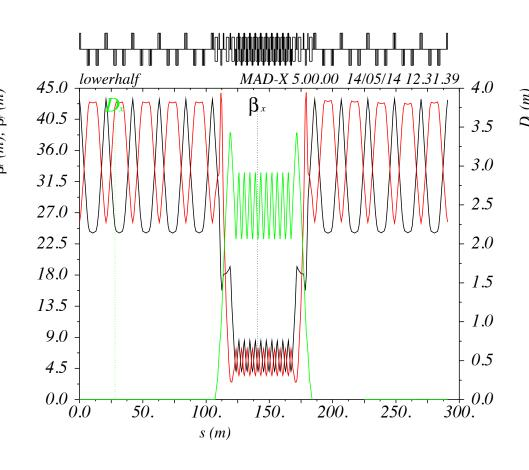
**Straight** – High beta values to minimise beam divergence (<  $0.1/\gamma$
