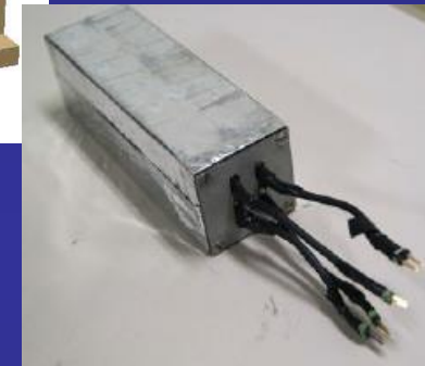
Prototype 2x2 crystal module wrapped with teflon and Al-mylar and 4 APDs.
