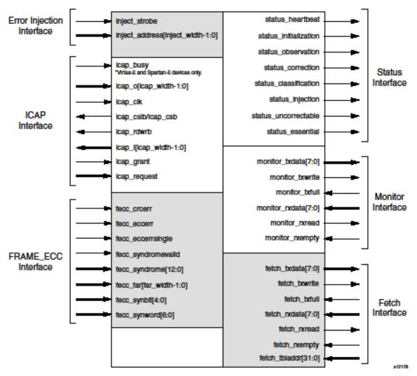
Figure 2-1: SEM Controller Ports
