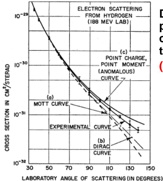
Determined proton RMS charge radius to be  $(0.7 \pm 0.2) \times 10^{-13} \text{ cm}$
