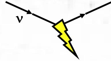
$$\frac{d\sigma}{d\cos\theta} = \frac{G_F^2 S}{\pi} \times \cos^2 \theta_{\text{Cabibbo}} \times (\xi_{\text{mass}}) \times \left( g_V^2 (1 + \beta_e \cos\theta) + 3g_A^2 \left( 1 - \frac{\beta_e}{3} \cos\theta \right) \right)$$
