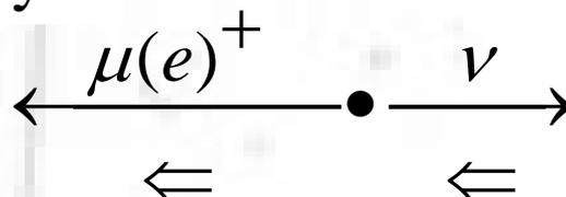
$$R_{theory} = \frac{\Gamma(\pi^+ \rightarrow e^+ \nu_e)}{\Gamma(\pi^+ \rightarrow \mu^+ \nu_\mu)} = \left(\frac{m_e}{m_\mu}\right)^2 \left(\frac{m_\pi^2 - m_e^2}{m_\pi^2 - m_\mu^2}\right)^2 = 1.23 \times 10^{-4}$$
