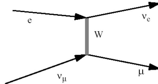
$$\begin{aligned} \sigma_{TOT} &\propto \int_{Q_{\min}^2}^{Q_{\max}^2} dQ^2 \frac{1}{(Q^2 + M_W^2)^2} \\ &\approx \frac{Q_{\max}^2 - Q_{\min}^2}{M_W^4} \\ \sigma_{TOT} &= \frac{G_F^2 (s - m_\mu^2)}{\pi} \\ &= \left[ \sigma_{TOT}^{(\text{massless})} \right] \left( 1 - \frac{m_\mu^2}{s} \right) \end{aligned}$$
