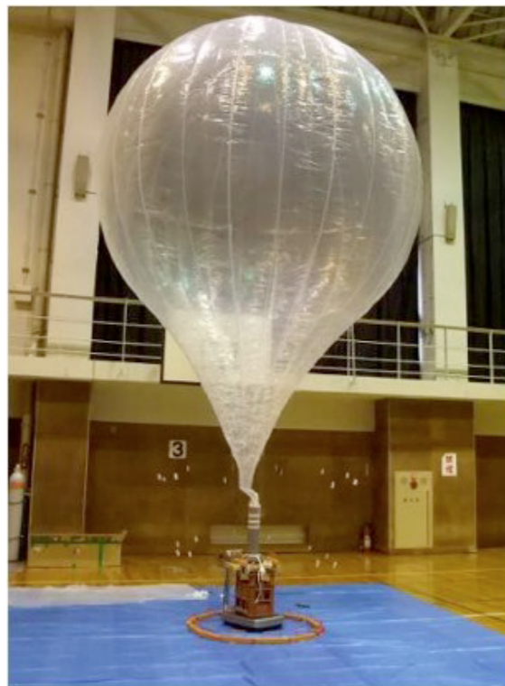
80 \mu\text{m} polyethylene test balloon
