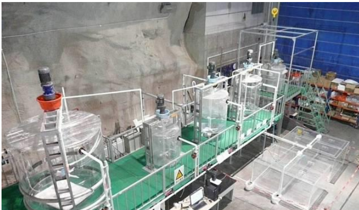
Gd-LS production Equipment and the process by Daya Bay
