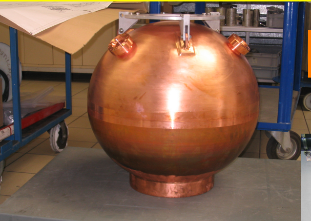
Low background detector d=60 cm p=10 bar
