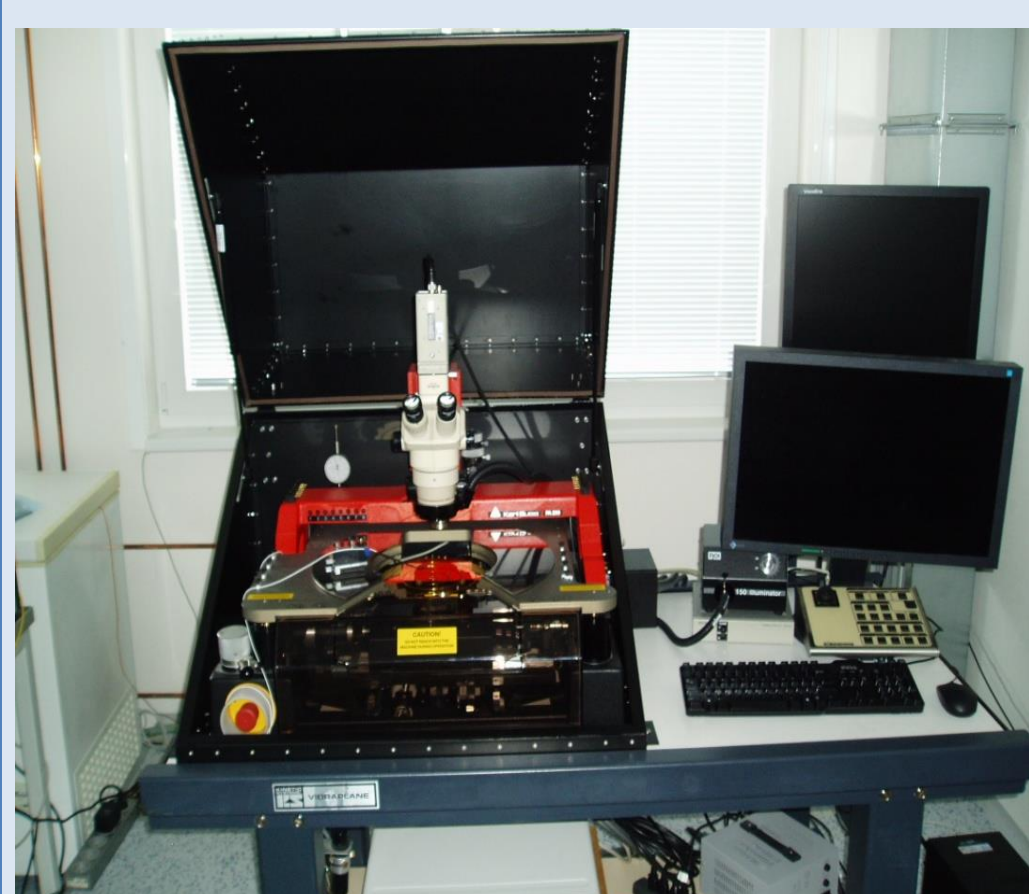
Semi-automatic probe-station KarlSuss PA200 in Prague Peltier module for cooling the manual probe-station chuck.
