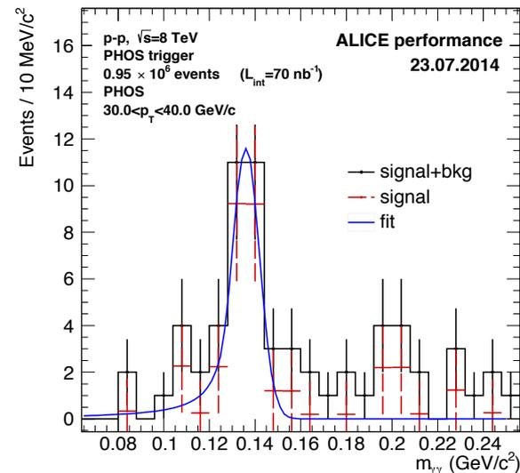
Neutral pion can be measured up to 40 GeV/c with PHOS trigger!
