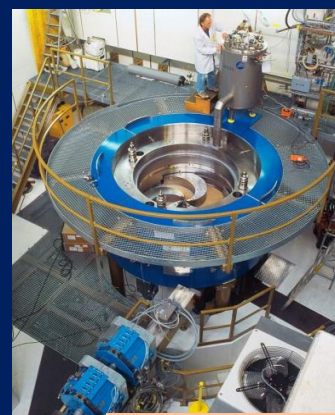
Example PSI Switzerland, Comet synchrotron 250 MeV
