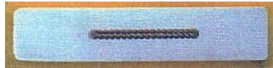
40 wires in a cable, surrounded by pure aluminium
