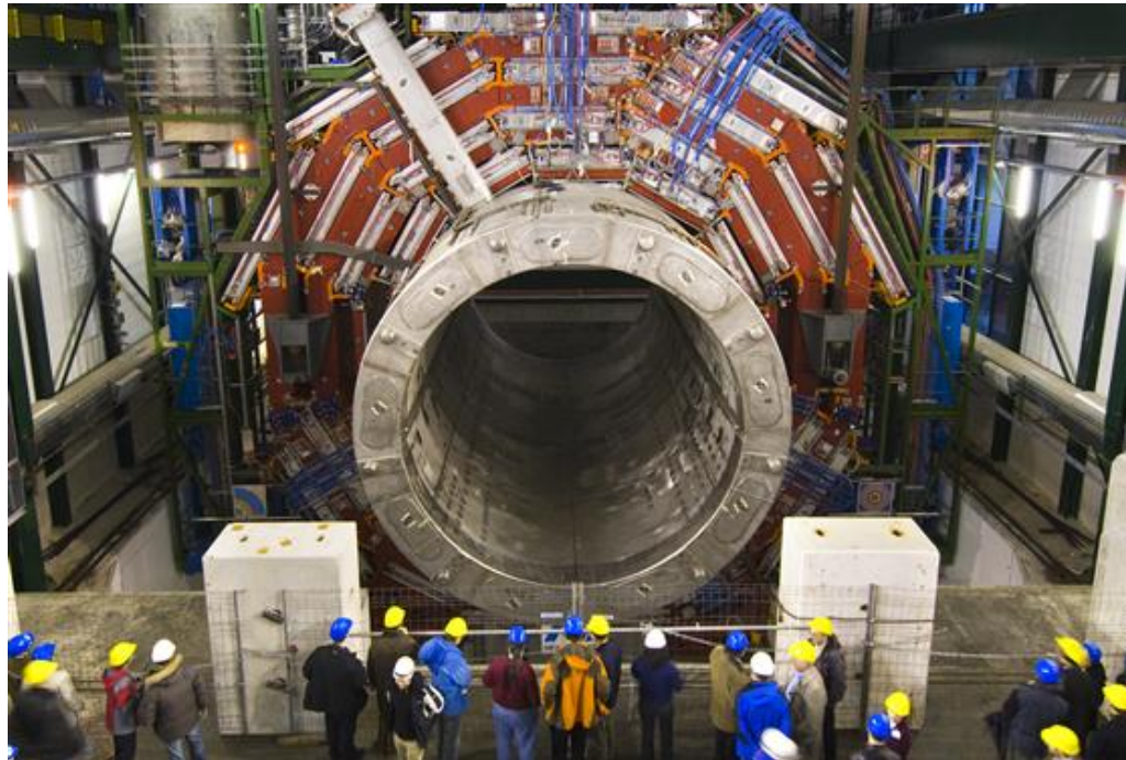
4 T CMS magnet completed and being installed in the cavern (2007)
