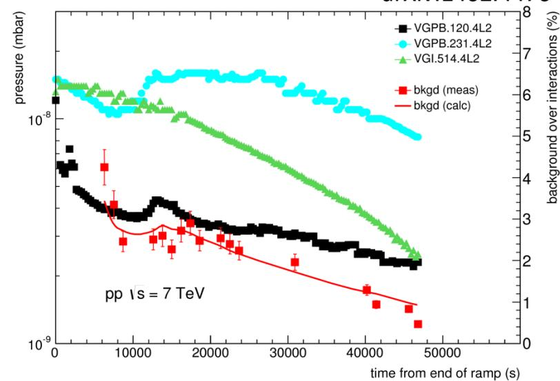
Pressure measured in Long Straight Section 2 (LSS2)
