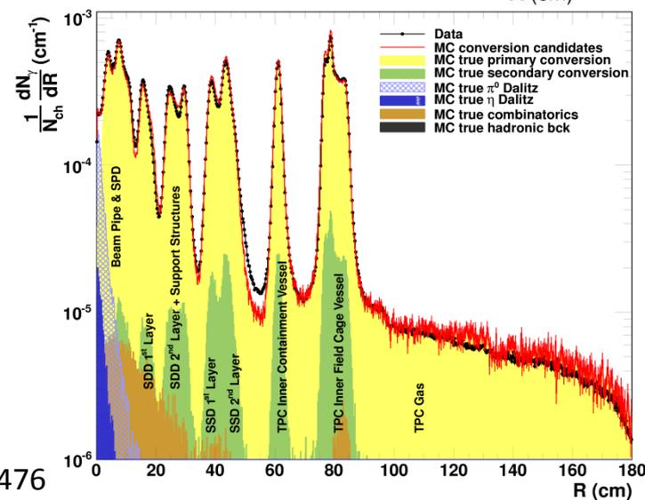
The integrated detector material for  $R < 180$  cm and  $|\eta| < 0.9$  amounts to a radiation thickness of  $11.4 \pm 0.5\% X_0$  and results in a conversion probability of about 8.5%.
