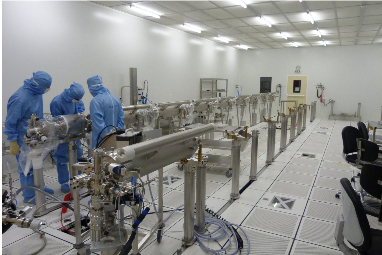
XM-1 cavity string in IS04 Clean Room (final leak test)
