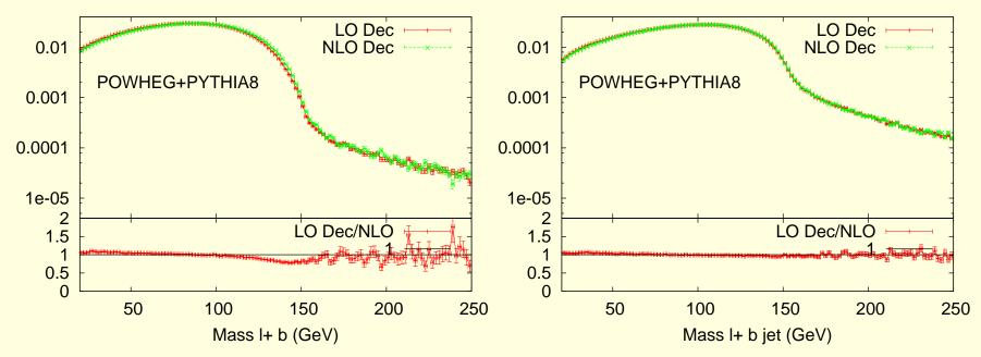
Effect of different fragmentation behaviour shows up in  $M_{l+b}$ , but not in  $M_{l+b \text{ jet}}$ .
