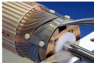
A close-up of the lower part of a 13kA current lead. Credit: CERN
