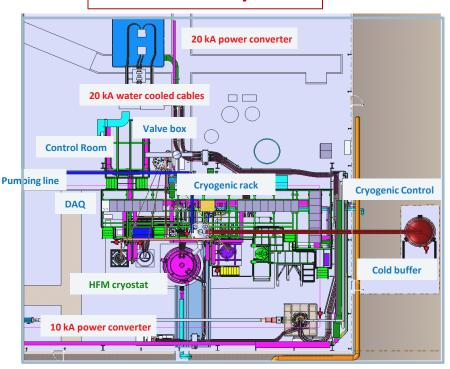
2 operational vertical cryostats @ 20 kA @ 1.9 K
