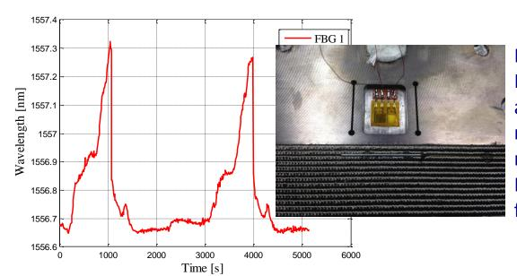
FBGs recoated with epoxy and PMMA have been selected and arranged in 4 arrays of 20 meters length in order to monitor the homogeneity of the Helium gas temperature in the first prototype of SC – Link.
