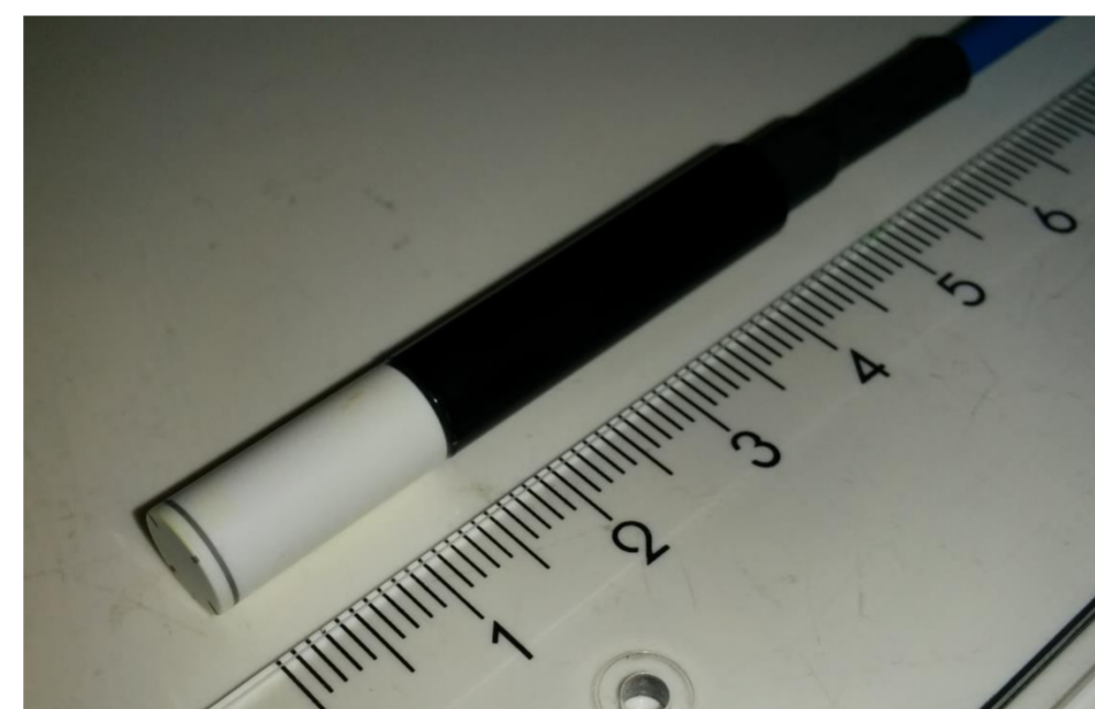
PTW Micro Diamond Sensitive area Radius: 1.1 mm Thickness: 1 μm
