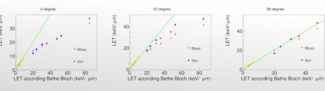
In the measurements at the angles 0° and 60° the predicted values by the Bethe-Bloch formula are only reached in the lower LET range. It is the range, where the per pixel energy deposition is below the saturation level for each pixel. For the measurement at 90° hardly any pixel exceeds the saturation level. Thus the measured LET resembles the theoretically calculated one.
