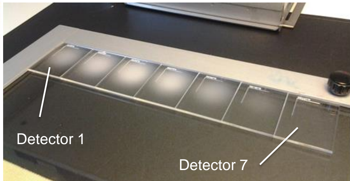
Beam shape marked in the CR-39 due to track overlap
