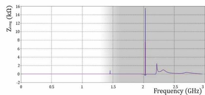
Simulated Z<sub>long</sub> of the cylindrical RP without ferrite and with zero gap between the detector housing and the flange
