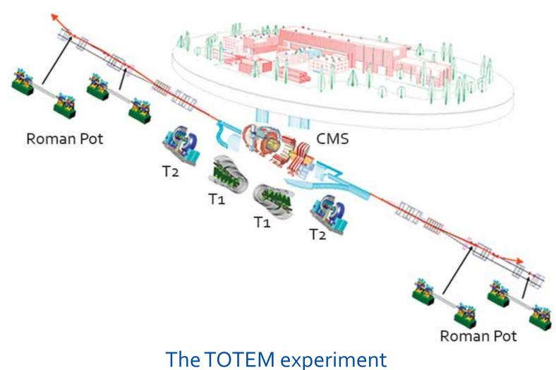
The TOTEM experiment was designed to measure the total proton-proton cross section and to study elastic and diffractive scattering at the LHC energy. In order to achieve a 2 % precision for the total cross-section using the Optical Theorem, one needs to be very close to the outgoing beam; this is done using Roman Pots.
