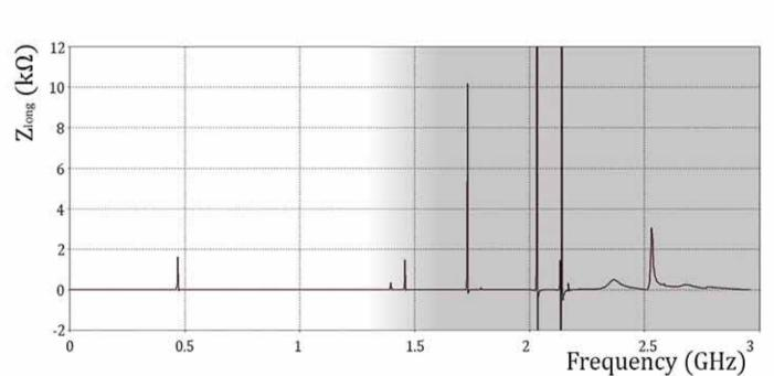
Simulated  $Z_{long}$  of the cylindrical RP without ferrite and with a realistical gap (2.5 mm) between the detector housing and the flange
