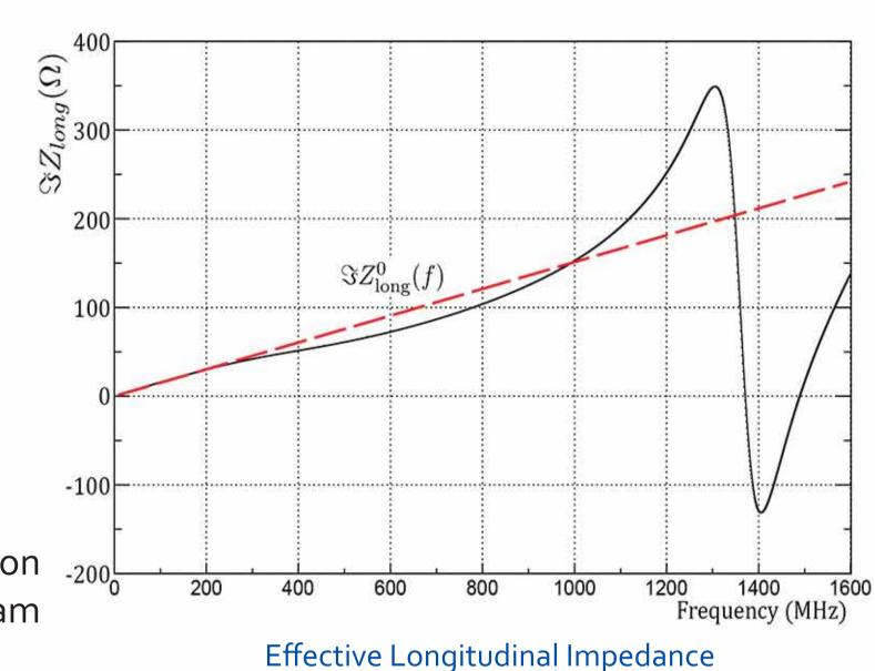
A charged beam perturbs its surroundings creating an electromagnetic field (wake field) that affects other charged particles.
