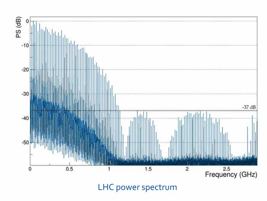
When the beam is passing through a cavity, part of its energy is dissipated on its walls, hence producing heat. The amount of heat produced depends on the characteristics of the cavity and of the beam power spectrum: in the LHC the heat is produced mainly by resonances below ~1.2 GHz.
