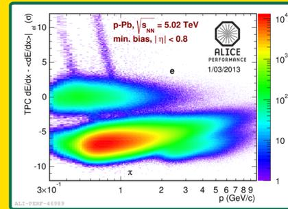
In the TPC, charged particles are identified via their specific energy loss  $dE/dx$  in the drift gas. The TPC  $dE/dx$  is shown as deviation from the expected energy loss of electrons, normalized by the  $dE/dx$  resolution. Due to overlapping  $dE/dx$  bands from kaons, protons and deuterons, a large hadron contamination is persistent. Here, TOF information is used to reject kaons and protons.
