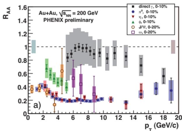
Measured nuclear modification factors for direct photons and various mesons by PHENIX detector at RHIC *a*.
