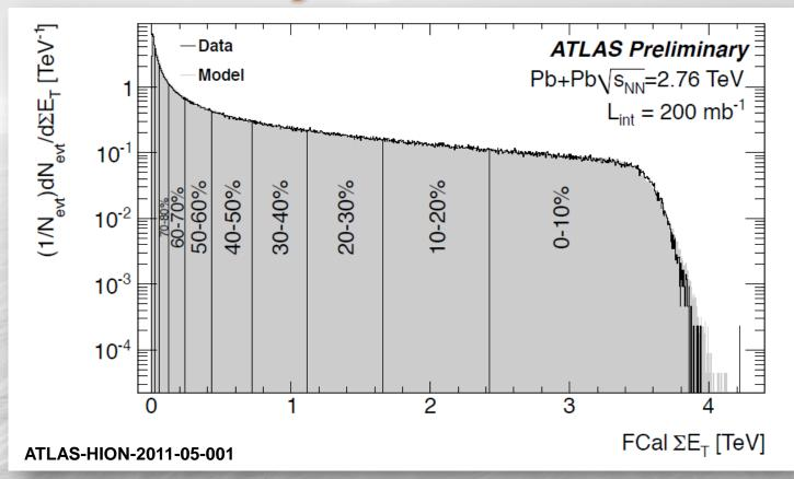
Based on FCAL energy (3.2< $|\eta|$ <4.9), Glauber model MC and p+p data @  $\sqrt{s}$ =2.76 TeV. MB selection efficiency 100% ± 2% efficiency
