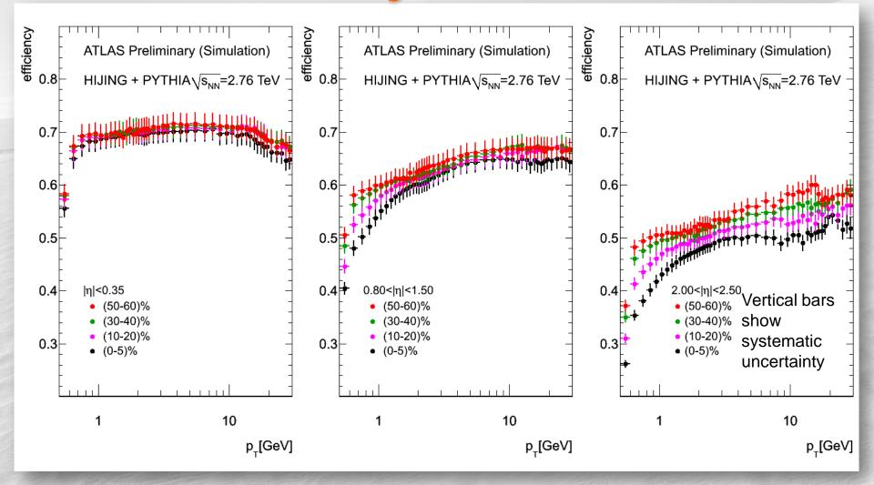
Efficiency based on the PYTHIA events embedded in HIJING MC. Loss at higher  $\eta$  is due to very restrictive cuts used in the analysis
