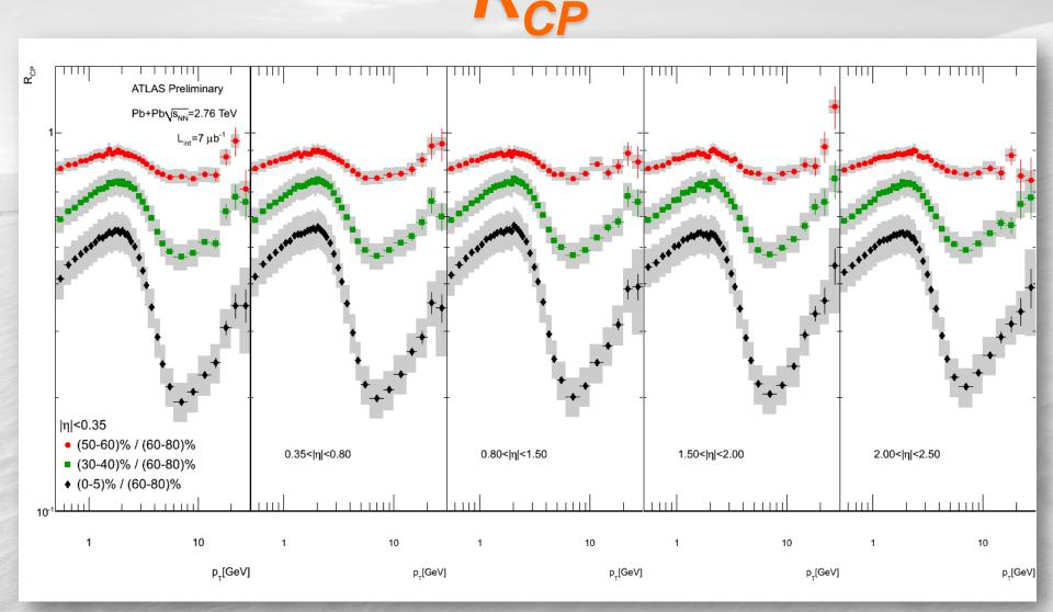
Central-to-Peripheral Nuclear Modification Factor. For the main result ATLAS uses (60-80)% centrality bin as the denominator.
