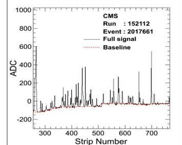
Fig. 2 shows an example of baseline reconstruction at high multiplicity in the presence of a deformation caused by highly ionizing particle. Shown in black are the ADC distribution over the 768 strips of a module. Shown in red is the corresponding reconstructed baseline that is subtracted before performing zero suppression.
