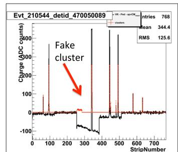
Fig. 1 shows the behavior of the standard zero suppression algorithm in case of baseline deformation. Shown in black is the ADC distribution over the 768 strips of a module. The corresponding reconstructed clusters are shown in red.
