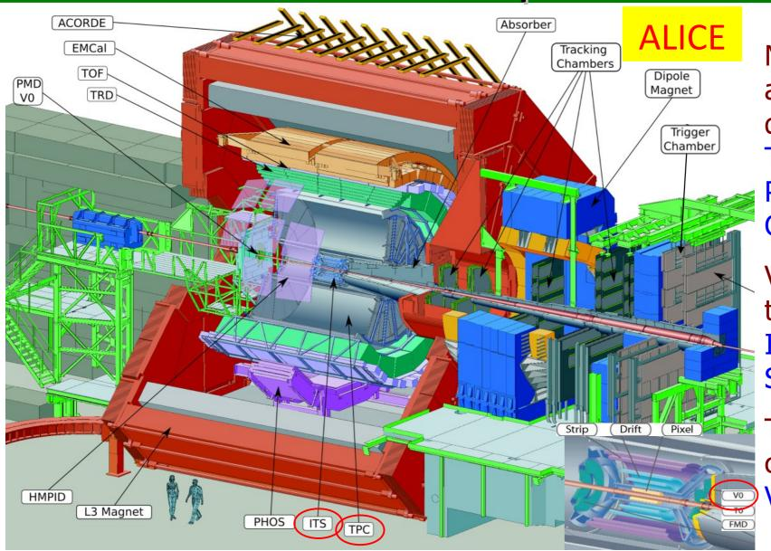
Main tracking and PID detector:
