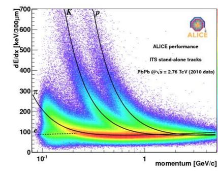
$dE/dx$  of charged particles vs momentum measured by the ITS standalone in Pb-Pb collisions at 2.76 TeV. The solid lines are a parametrization[5] of the detector response based on the Bethe-Bloch formula.
