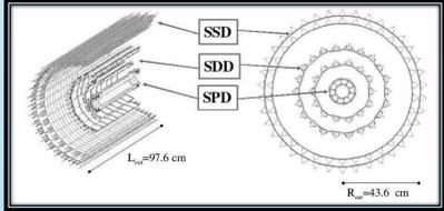
6 cylindrical layers of silicon detectors:
