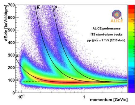
$dE/dx$  of charged particles vs momentum measured by the ITS standalone in p-p collisions at 7 TeV. The solid lines are a parametrization[5] of the detector response based on the Bethe-Bloch formula.
