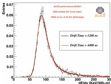
$dE/dx$  distribution for 1 typical SDD module in 2 different drift time intervals during Pb-Pb 2010 run. The  $dE/dx$  is in  $\text{keV}/300\ \mu\text{m}$  after applying all the needed calibrations and corrections. Fits with a convolution of a Landau and a Gaussian function are also shown. This plot demonstrates the effectiveness of the correction applied to account for the drift time dependence of the raw ADC counts per cluster.
