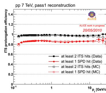
Efficiency of the track prolongation from the TPC to the ITS for p-p data at 7 TeV.
