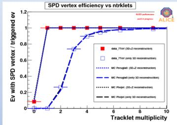
Primary vertex efficiency with SPD tracklets: as a function of the multiplicity for data and Monte Carlo in p-p at  $\sqrt{s} = 7$  TeV.
