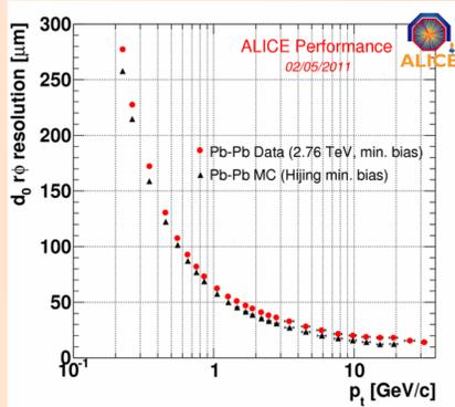
Transverse impact parameter resolution as a function of  $p_t$  for tracks reconstructed in minimum bias Pb-Pb collisions at 2.76 TeV.
