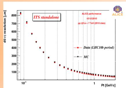
Transverse impact parameter resolution as a function of  $p_t$  for tracks reconstructed by the ITS standalone in p-p collisions at 7 TeV. ITS Standalone allows tracking for very low momentum particles.
