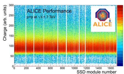
$dE/dx$  distribution for all the 1698 SSD modules in pp collisions at 7 TeV. Each bin is a Landau-Gaussian convolution distribution. This plot shows the uniformity and stability of the charge collection among all the modules.
