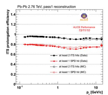
Efficiency of the track prolongation from the TPC to the ITS for Pb-Pb data at 2.76 TeV.
