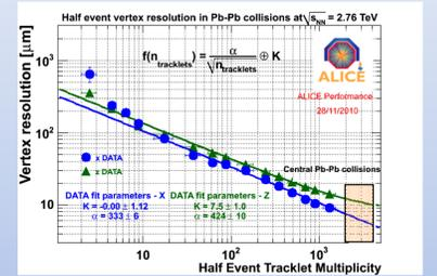
Primary vertex reconstructed with tracks in Pb-Pb data at 2.76 TeV per nucleon pair. The track sample is randomly divided into two. The primary vertex is reconstructed for each sub-sample. The residual distribution of the 2 vertices is fitted with a Gaussian and  $\sigma/\sqrt{2}$  is taken as the vertex resolution. The resolution is extrapolated for most central (5%) Pb-Pb collisions.
