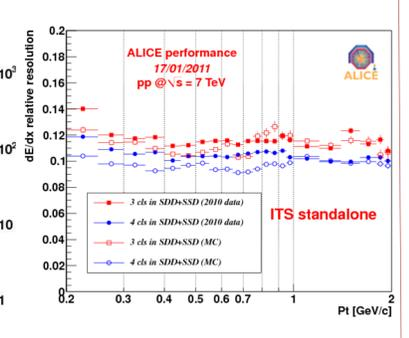
$dE/dx$  resolution for charged particles vs momentum measured by the ITS standalone, in p-p collisions at 7 TeV.
