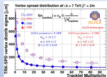
Primary vertex reconstructed with tracks and with SPD tracklets only in 7 TeV p-p data. The asymptotic limit of the vertices reconstructed with tracks (filled markers) estimates the size of the luminous region.
