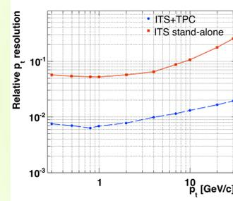
Comparison of the  $p_t$  resolution for the standard ITS + TPC tracking and for the ITS standalone tracking as a function of  $p_t$  [4]. The momentum resolution of the ITS standalone allows efficient tracking of very low momentum particles. It depends on the length of the lever-arm and the number of points per track.
