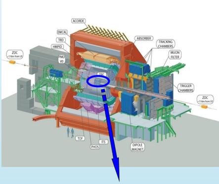
The ALICE[1] detector consists of a central barrel part, which measures hadrons, electrons, and photons, and a forward muon spectrometer. The central part is embedded in the large L3 solenoidal magnet (max field 0.5T). The Inner Tracking system (ITS) in conjunction with the Time-Projection Chamber (TPC) provide track finding, charged particle momentum measurement, particle identification and vertex determination in the pseudo-rapidity region  $|\eta| < 0.9$ .
