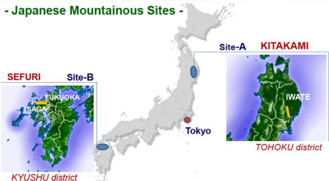
"Issues that could lead to particularly serious difficulties for the Sefuri site are that the route passes under or near a dam lake, and that the route passes under a city zone. Also, the lengths of access tunnels are longer for the Sefuri site than for the Kitakami site leading to a large merit for the latter in terms of cost, schedule, and drainage."
