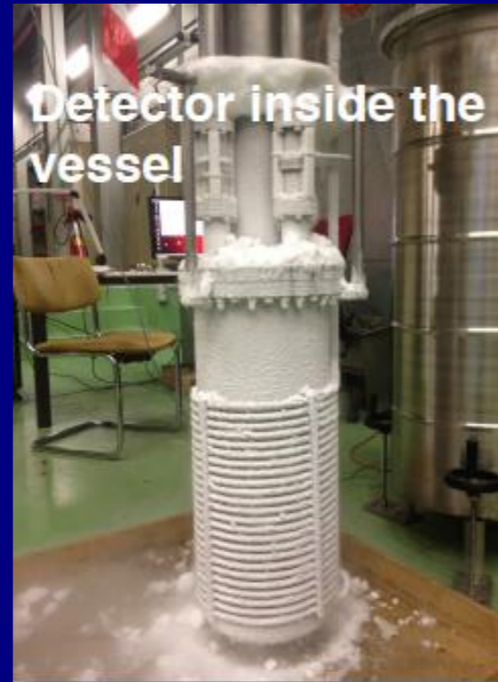
10x10x20 cm LEM-anode fast test setup
