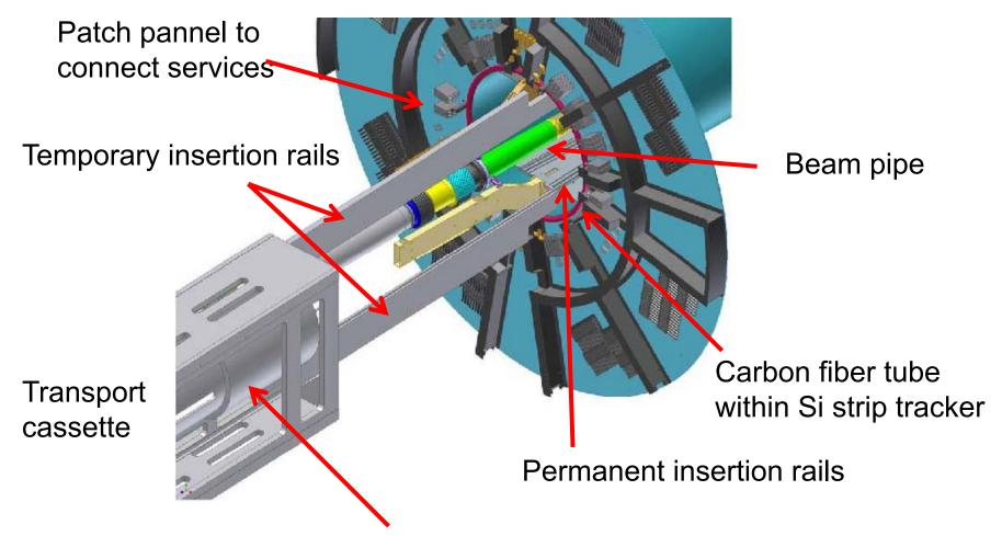
System supply tube – detector – supply tube fully assembled and connected
