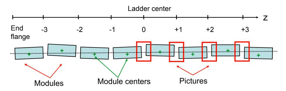
Take pictures of region where modules are facing each other. Connect modules positions from center outward For BPix a ladder is not a mechanically independent object There are no fiducial points on a ladder
