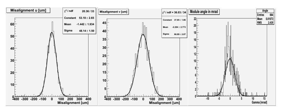
Shown is position and angle of module w.r.t. ideal position on ladder Measured misalignments: 50µm in u=r-phi (gauss)
