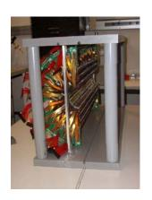
Clearance test with real detector and mockup rail system Clearance between left/right halfs:1mm!
