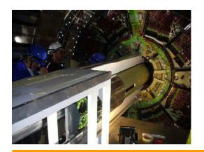
Insertion test with ,commissioning system': true mechanical structure, prototype supplytube, only one sector (1/32) equipped with modules
