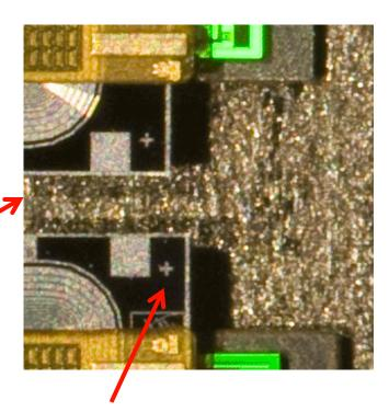
Alignmnet mark on active material, one at each corner Size: 100µm
