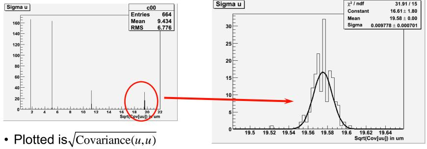
• Error is z-dependent: each peak corresponds to position  $\pm n$  on the ladder. It gets bigger further away from the ladder center
