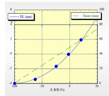
Path length variation as a function of wiggler field and maximum transverse displacement of the trajectory
