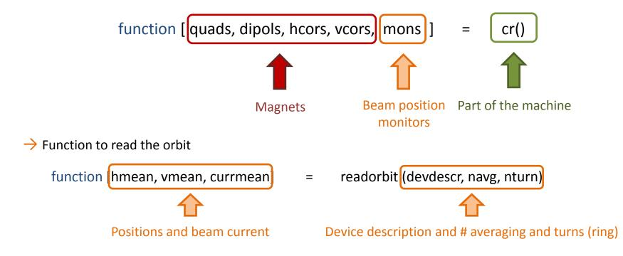
→ Function to automatically read and write the currents in the magnets
