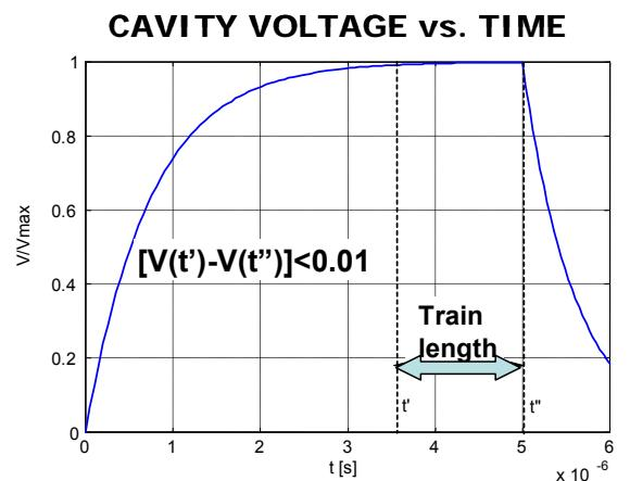
In **CLIC** the linac pulse ( $\sim 140 \mu$ s) is generally much longer than the cavity filling time even in case of cavity with high loaded Q (that means higher efficiency structures).
