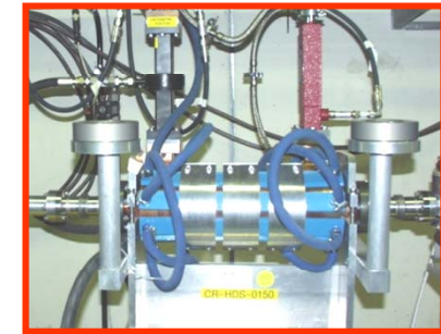
RF deflectors for injections in the rings
