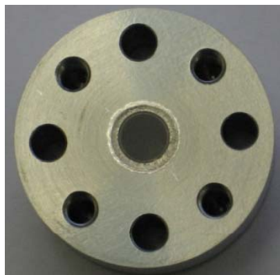
0.500 ± 0.005 mm thick CVD diamond window \epsilon_r \sim 6 at 30 GHz Braze at CERN (S. Mathot)
