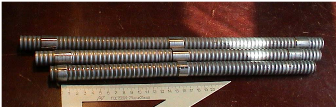
Main parameters and photo of Bragg resonators with shift of corrugation phase
