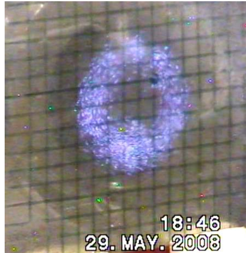
Wavebeam visualisation after the test cavity ( TE_{01} mode)
