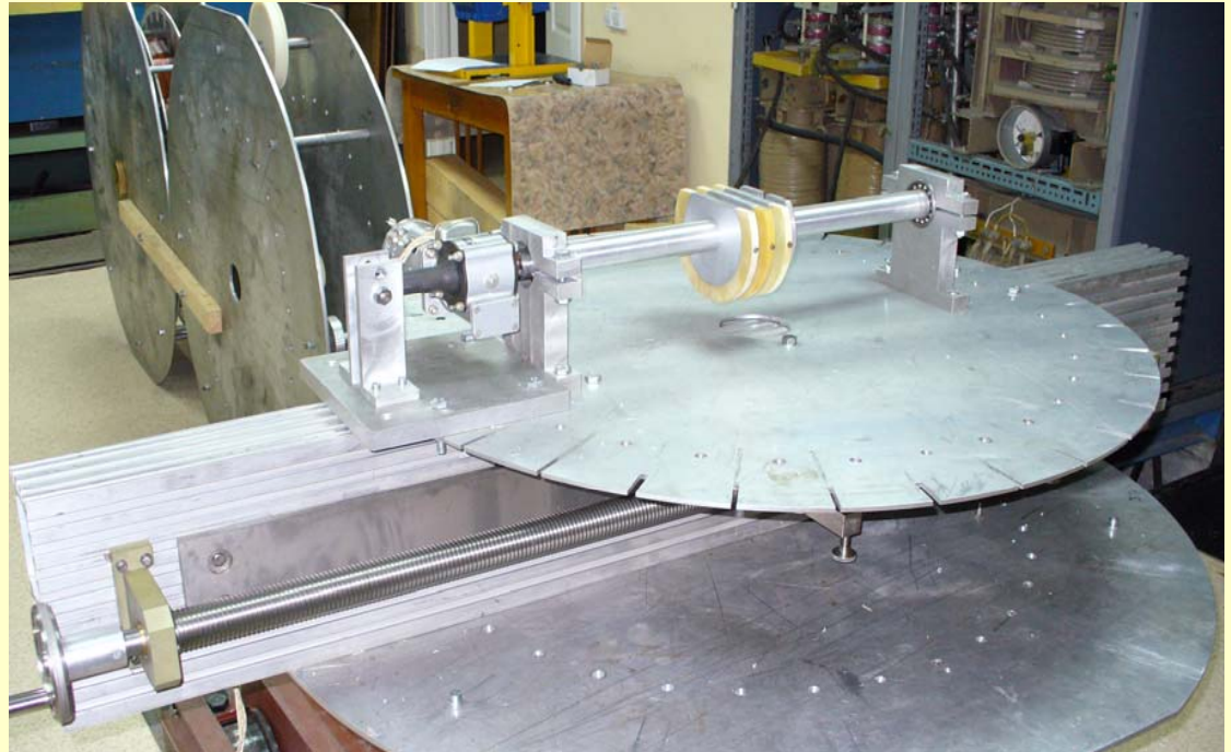
Tool for coil winding into iron yoke slots with help of one wire piece
