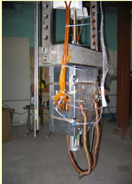
Method of wiggler fastening inside cryostat
