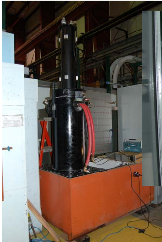
Klystron and solenoid and HV Transformer
