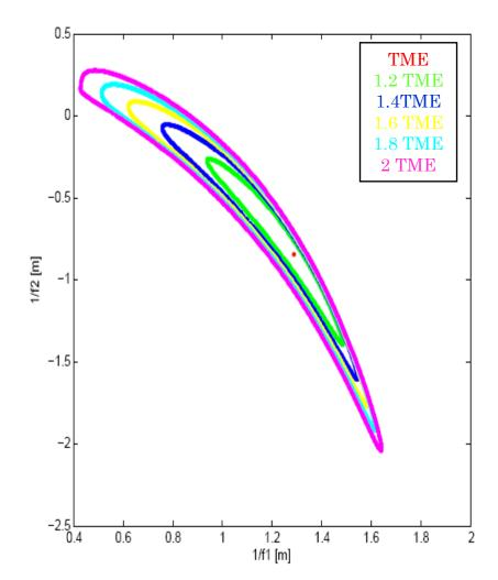
A possible configuration for the  $l_{l}$ ,  $l_{2}$ ,  $l_{3}$  for low chromaticity (and small focusing strengths) at both the planes is chosen for the TME:
