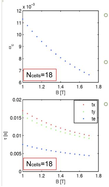
Momentum compaction factor (up)  $a_{o} = \frac{1}{C} \sum_{i} \langle D \rangle_{i} \, \theta_{i} = \frac{1}{C} N_{d} \left( 2\eta_{od} + 7 \, \frac{L_{d}^{2}}{12 \, \rho} \right) \frac{L_{d}}{\rho}$   $a_{o,TME} = \frac{12 \, \theta^{3} \rho}{C}$
