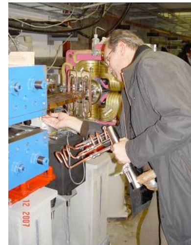
Regular absorbers of 26kW for PETRA-III project
