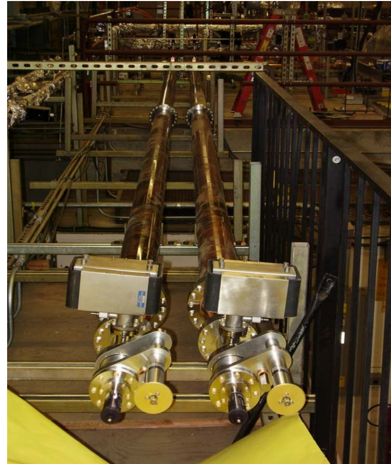
The ASTA pulse compressor with variable delay delay-lines( Miller cup)
