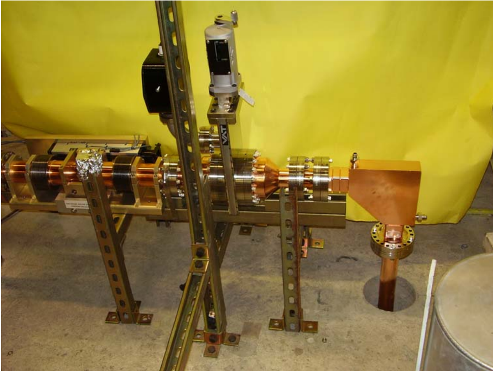
The uncompressed arm has a variable phase shifter and a gate valve
