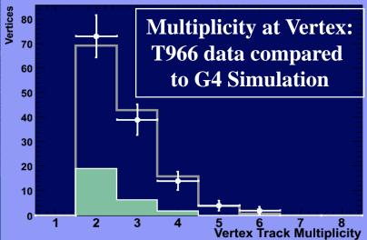
Extrapolate 3.3 cm upstream from first Si pixel layer:  $\sigma_{z vtx} = 230 \ \mu m$
