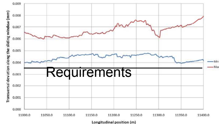
100 simulations of the Modules alignment along 400m WPS offsets errors at 5 \mu\text{m}
