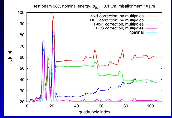
$\rightarrow$  Dispersion Free Steering works in the collimation section.
