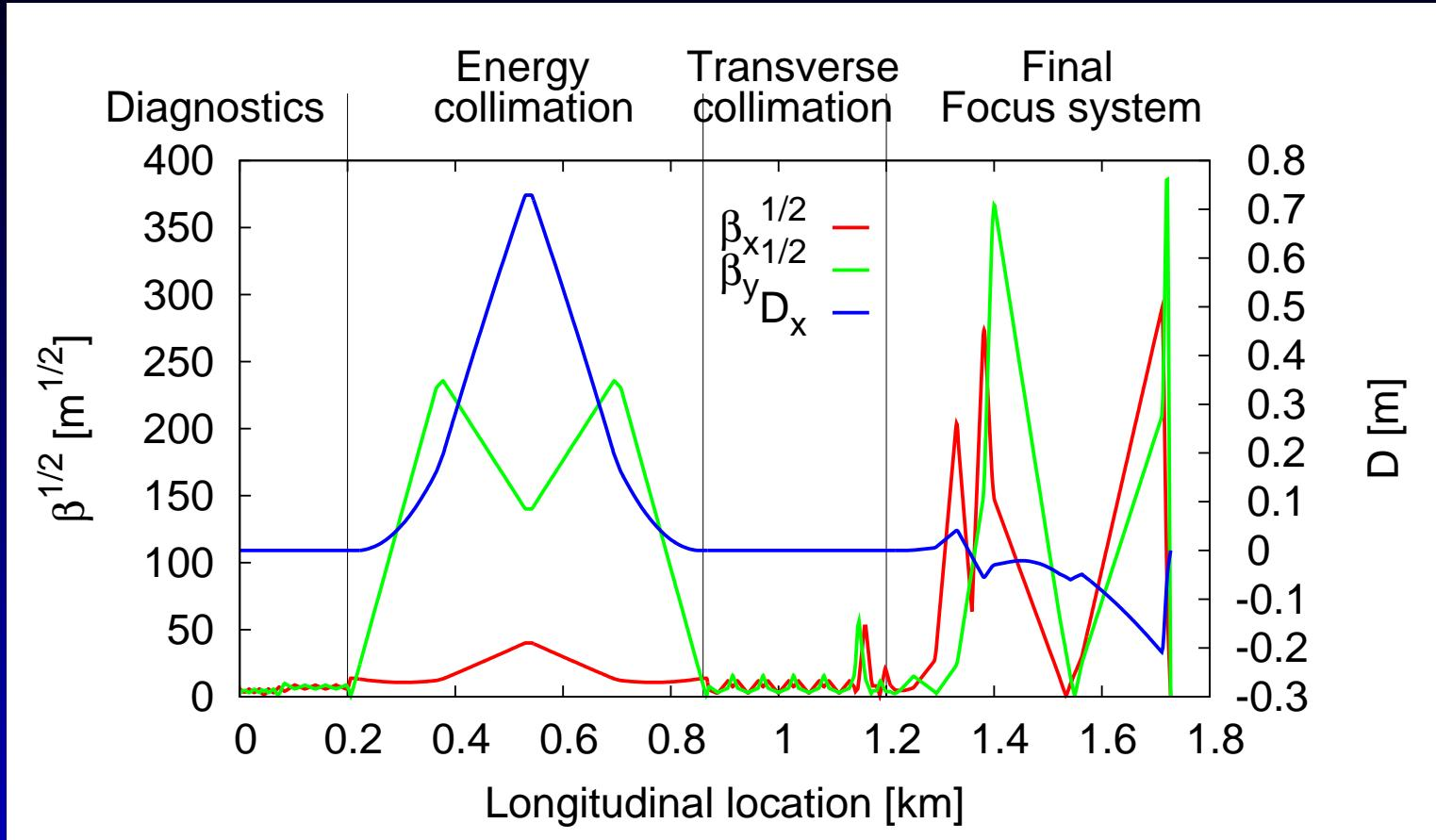
Collimation section can be scaled by a factor 2.
