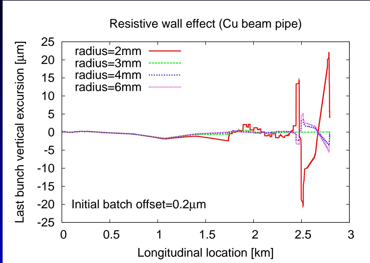
Simulations by G. Rumolo and D. Schulte suggest a beam-pipe radius of 8mm
