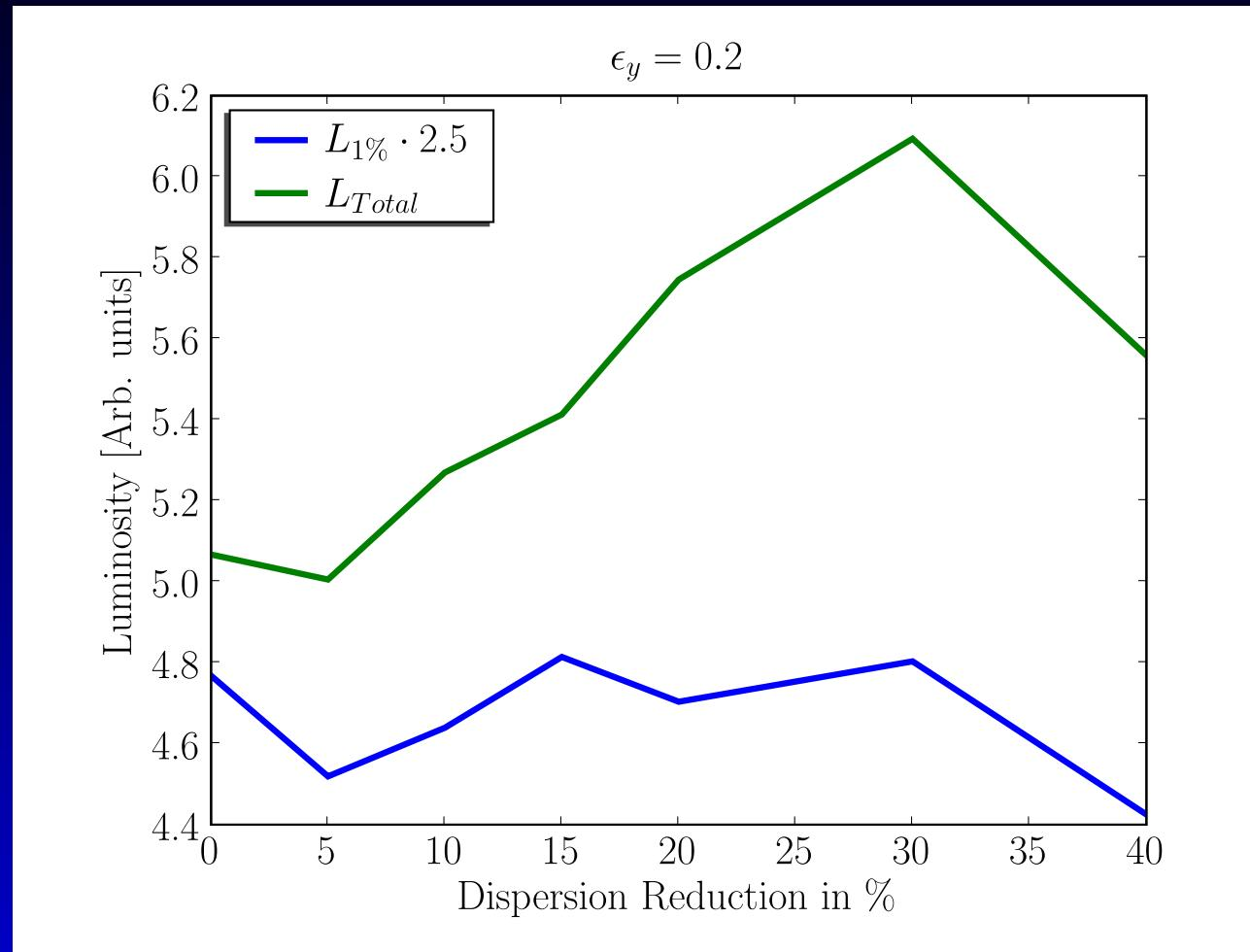
→ With the current beam parameters further reductions of IP beam size do not increase peak luminosity
