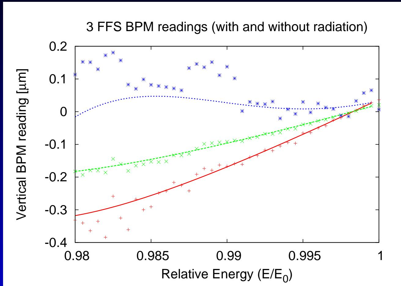
The FFS is the most complex section. Rather than align the FFS, general tuning algorithms must be used.
