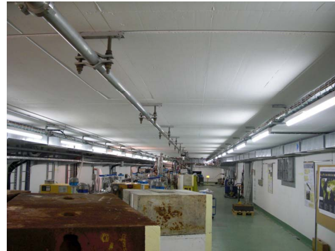
UV Laser transport under vacuum
