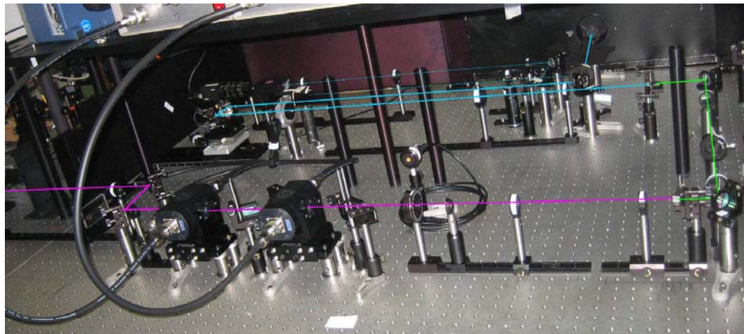
Laser-room table with pulse picker and conversion crystals
