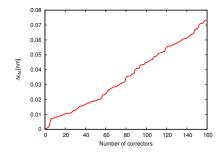
• Calibration error and corrector strength noise (indep. from pulse to pulse) cause little  $\Delta \epsilon_N$  (emittance stated in [10<sup>-3</sup> nm]).
