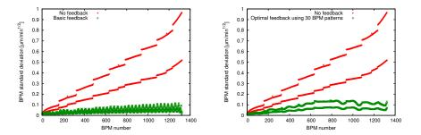
Improved trajectory control requires that the 30 most important BPM patterns are used to predict the less important. A modified equation gives a better solution:
