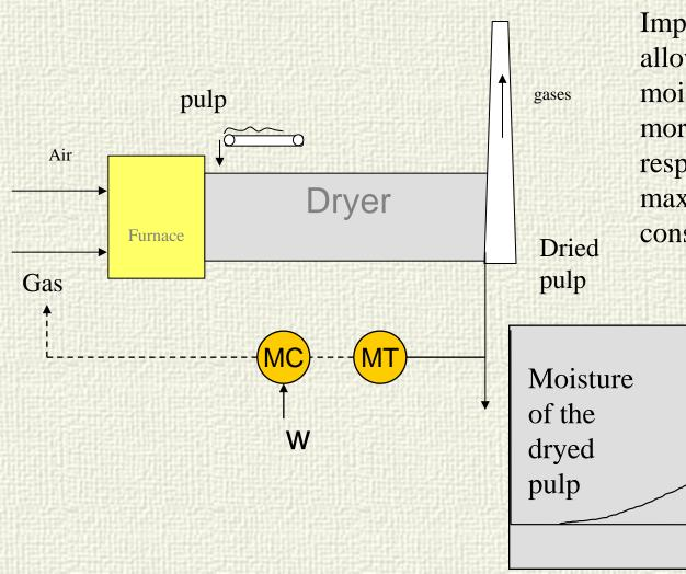
Improving control allows to move the moisture set point to a more profitable value, respecting the maximum moisture constraint
