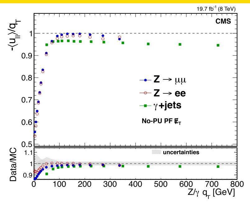
As noted before, NoPU MET algorithm sacrifices some of the MET response in exchange for improved resolution.
