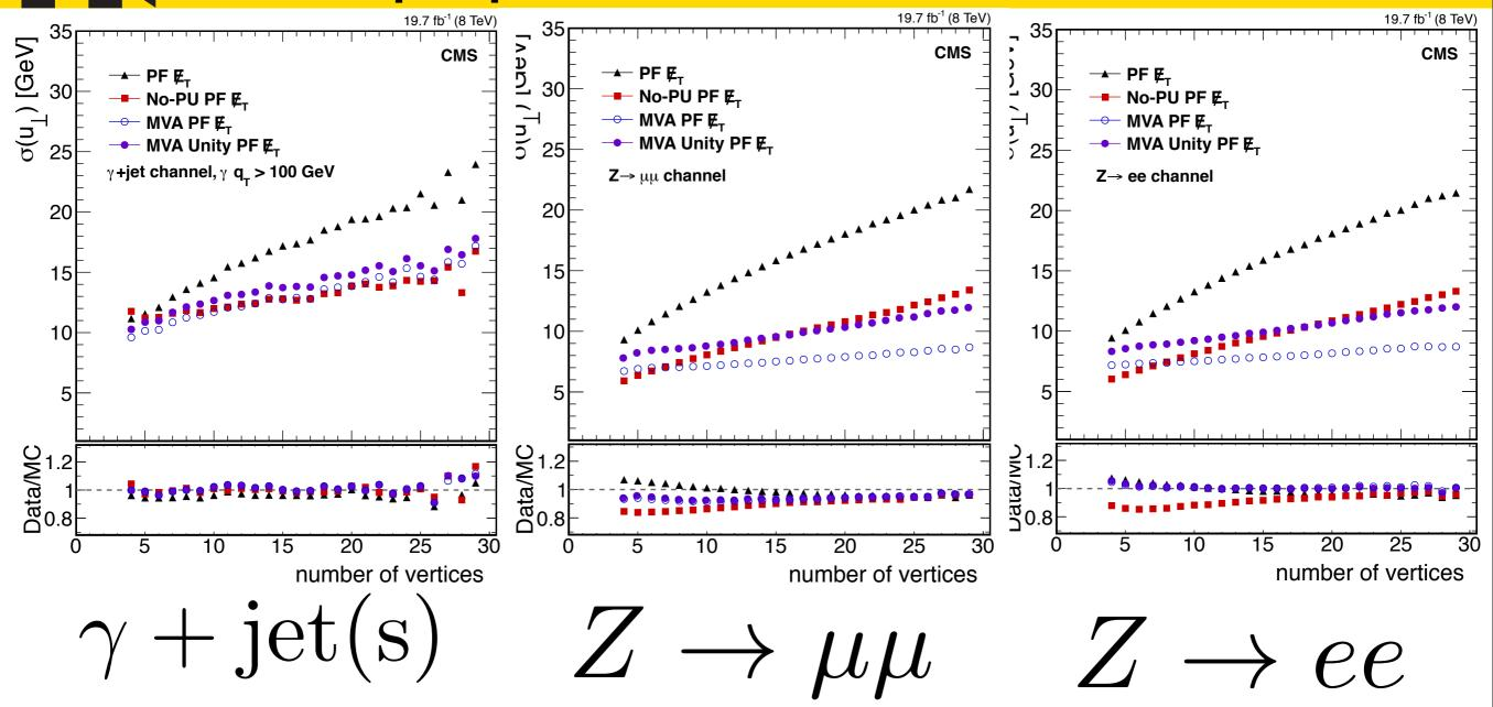
PU Mitigation algorithms greatly help with MET resolution degradation from Pileup
