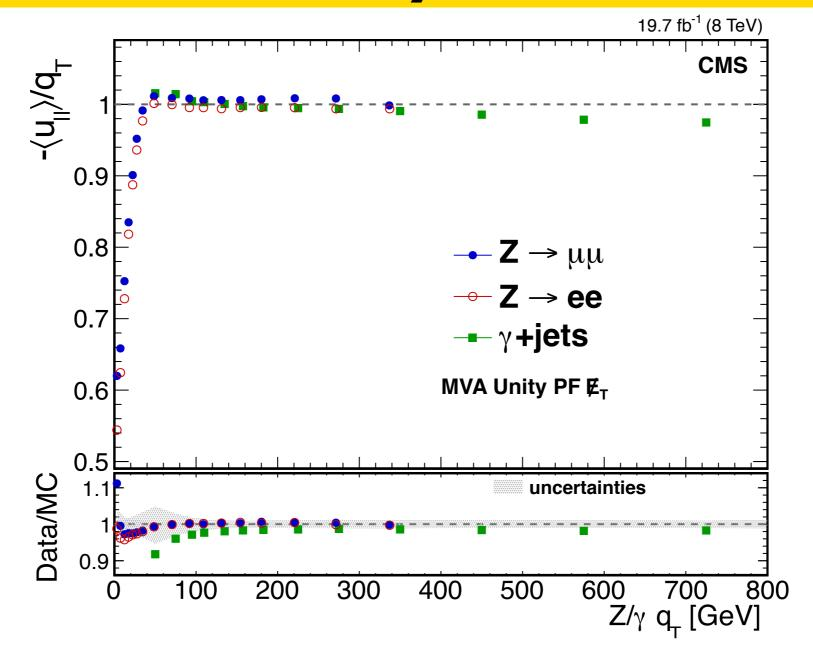
As shown on last slide, **without Unity** response, MVA MET algorithm loses MET response
