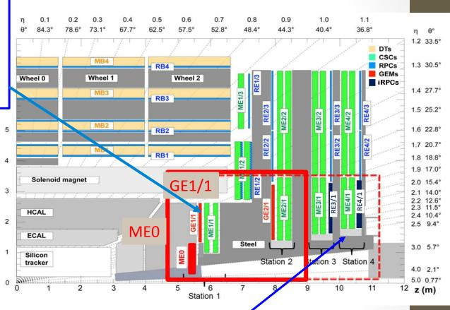
Enhance region without redundancy 1.6 <  $|\eta|$  < 2.4 with **maximum rate.** Technology = GEM (GE2/1) and improved high-rate RPC (RE3/1 and RE4/1)
