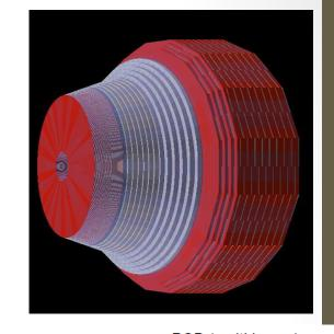
PCB (multi layers) Shieldina (1600 µm) Silicon wafer (thickness 500 µm) Back HCAL as HE re-build 5λ with increased (0.325 mm)transverse granularity Stainless steel plate (500 µm) Lead absorber  $(2000 \mu m)$ Cooling plate (3000 µm) Asic packaging (BGA)  $(1700 \mu m)$
