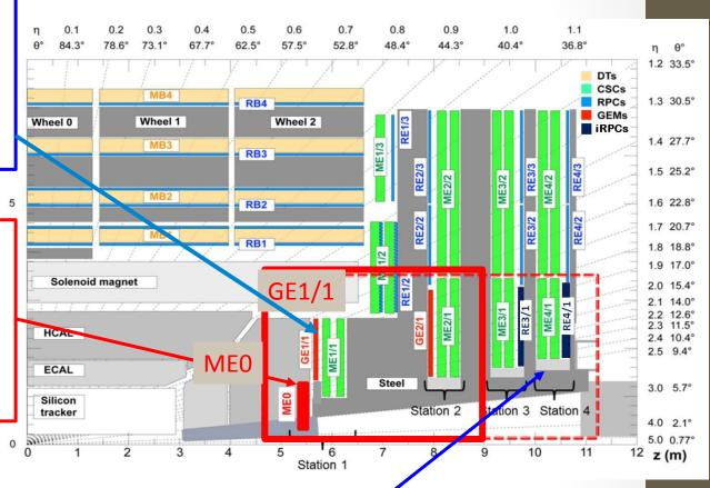
Enhance region without redundancy 1.6 <  $|\eta|$  < 2.4 with **maximum rate.** Technology = GEM (GE2/1) and improved high-rate RPC (RE3/1 and RE4/1)
