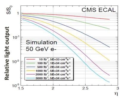
Many high rate testbeam campaigns, aging projections and simulations
