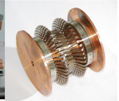
Deformable RF finger prototype
