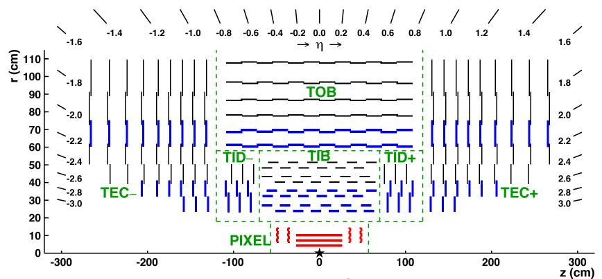
Pixel: 66M channels, 100x150 µm<sup>2</sup>
